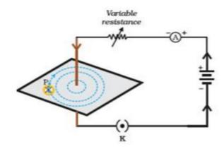
b) The strength of magnetic field due to a current-carrying straight conductor is inversely proportional to the normal distance between the conductor and the point where magnetic field is to be determined. So as the point as moved away the strength of the magnetic field goes on decreasing.
