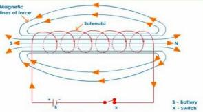
The field lines inside the solenoid are in the form of parallel straight lines. Which indicates that the magnetic field is the same at all points inside the solenoid. i.e. the field is uniform inside the solenoid.
